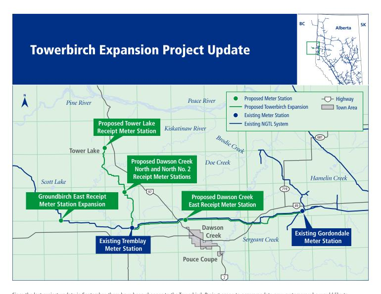
Since the last project update in September, there have been changes to the Towerbirch Project scope to accommodate new customers who would like to transport natural gas on the NGTL System. The meter station sites will include a skid-mounted meter-run building and instrument building and associated piping that will connect the customers to the natural gas pipeline. The project will now include:
