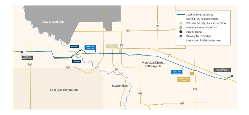
Construction of the new 20-inch pipeline loop requires a watercourse crossing at the Beaver River so NGTL will use a horizontal directional drill (HDD) to safely bore a path under the watercourse for the pipeline loop.
