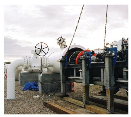
In-line inspection tools are equipped with hundreds of electronic sensors that inspect the quality of the pipeline inside and out to identify even the tiniest crack, flaw or sign of corrosion.
