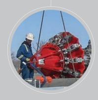
TransCanada's advancement of Electromagnetic Acoustic Transducer (EMAT) technology, a non-destructive in-line inspection tool that uses sound waves to detect defects in steel pipelines, has allowed EMAT to be used as an alternative to the hydrostatic testing of pipelines, eliminating impact to water sources and resulting in considerable cost savings. TransCanada continues our work on this important innovative initiative as part of our commitment to protecting the environment.
