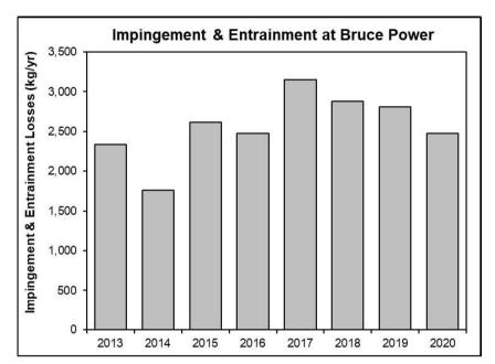
Figure 55: Total impingement and entrainment losses at Bruce Power (2013-2020) ,calculated using the HPI metric [R-103] [R-104]. Impingement was measured in all years. Entrainment was measured in 2013-2014 and estimated in 2015-2020 using a conservative approach.
