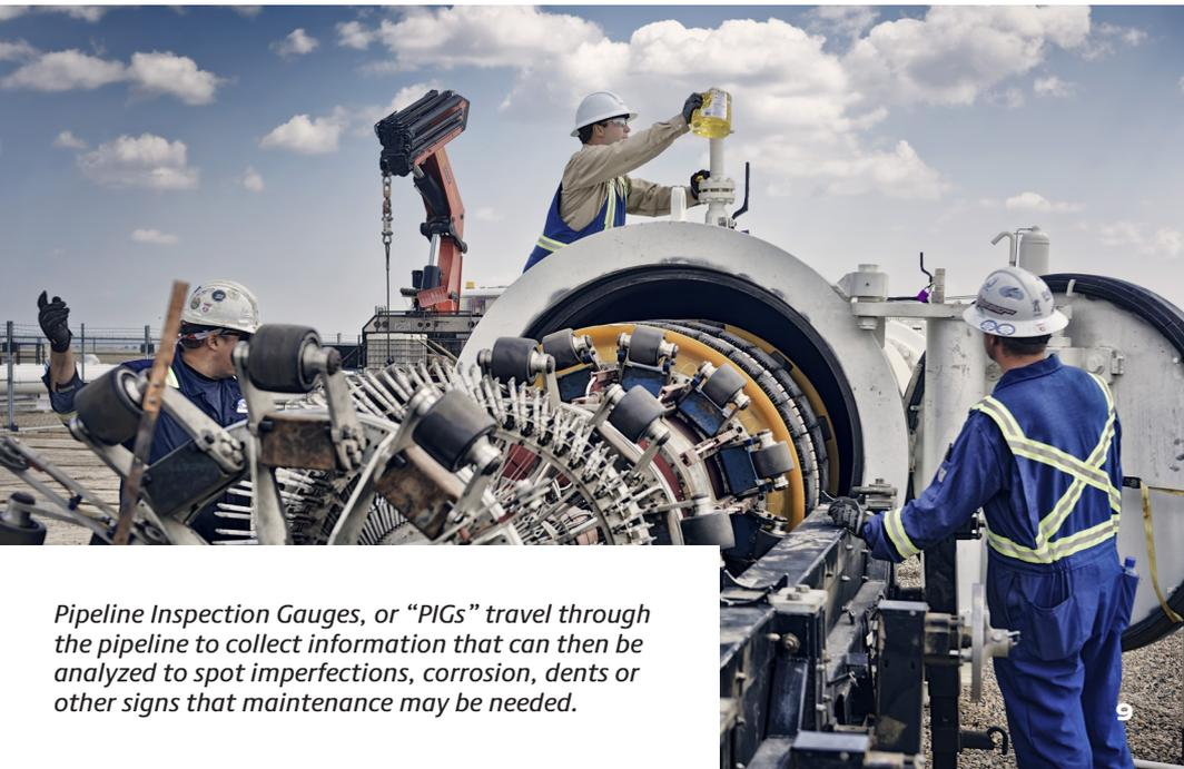
*Pipeline Inspection Gauges, or “PIGs” travel through the pipeline to collect information that can then be analyzed to spot imperfections, corrosion, dents or other signs that maintenance may be needed.*
