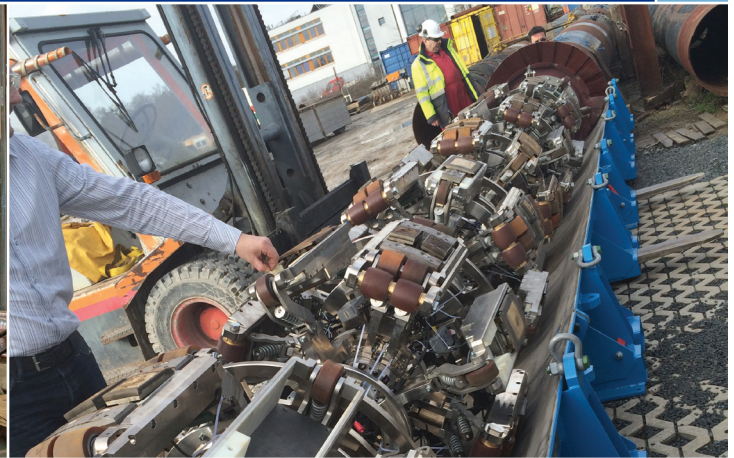
Smart pig modified with EMAT before its launch into the pipeline Photo courtesy of ROSEN
